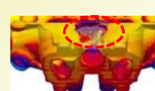
Examples of misrun and air entrapment detections ▲
