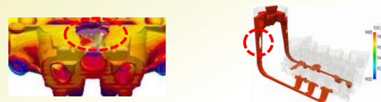
Examples of misrun and air entrapment detections ▲
